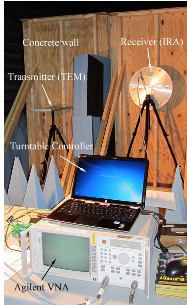
Figure 10. Equipment Used. The above photograph displays the equipment, as it was arranged in the Indoor Range. The transmitting and receiving antennas were located behind a concrete wall (framed by plywood, so the concrete is not visible in this image), and aimed along a path parallel to an adjacent wall (on the right, not shown). The Agilent VNA provided and received the radar signals, while the laptop was used to control the turntable and download radar data. The pale blue pyramids are the absorbing foam, surrounding the entire setup, and a stack of foam was placed between the antennas in order to cut down some of the interference between them.
